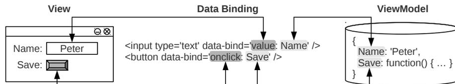
Figure 2: Data Binding between View and ViewModel
