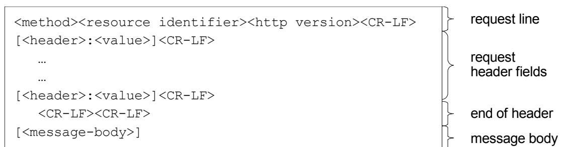
Figure 3-1: HTTP request format.
