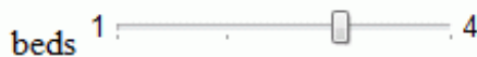
Figure 3.7.: HTML form example rendered in Opera 11. The <input type="range"> element is displayed as a slider. The minimum and maximum values on the left and on the right have been added using CSS.
