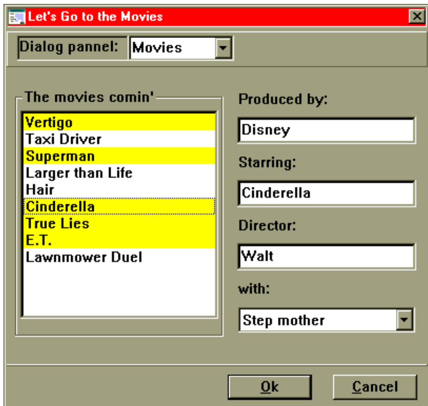
Figure 152. Let's Go to the Movies Sample: Movies This page show the drop-down style using a combo box.
