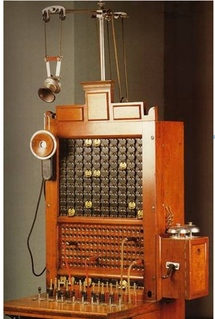
"Switchboard" with 100 ports
