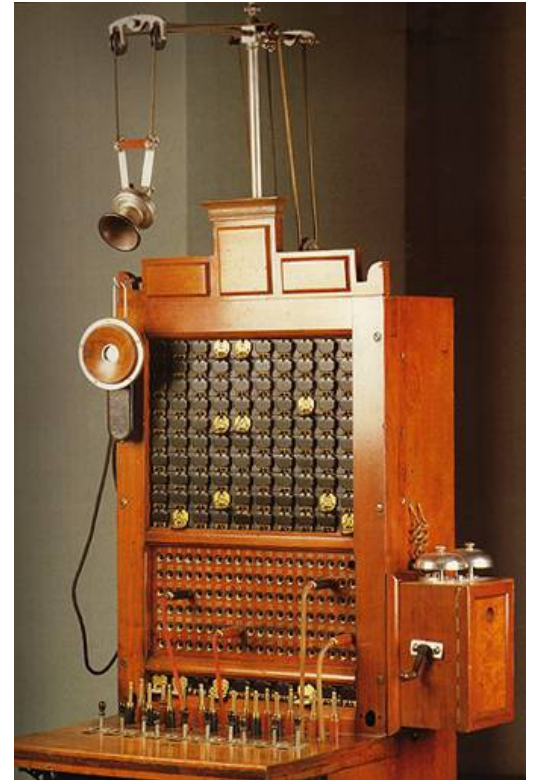
"Switchboard" with 100 ports
